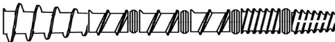
Figure 1. Schematic of extruder screw profile. Inlet starting on the left to discharge ending on the right. Screw element 1: inlet screw, single flight full pitch; 2: single flight, full pitch screw; 3: small steam lock; 4: single flight full pitch screw; 5: small steam lock; 6: Single flight, full pitch screw; 7: medium steam lock; 8: double flight, 1/2 pitch screw; 9: Large steam lock; 10: double flight, 1/2 pitch, cut cone screw.
